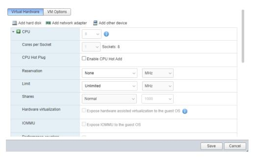
Alternatively, if the *CPU Hot Add* feature is enabled, ensure that the number of vCPUs assigned to the FortiAnalyzer VM is equal to the maximum number of licensed CPUs on the host.
